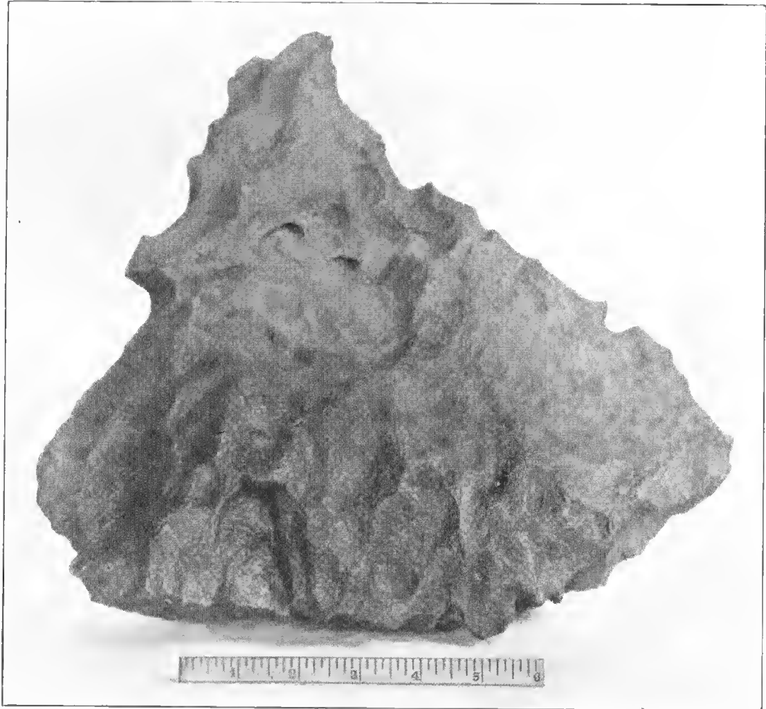
Fig. 2. Specimen of meteoric iron weighing 52½ lb. When found the darker area in the foreground was exposed to the air, the lighter portion being buried.
